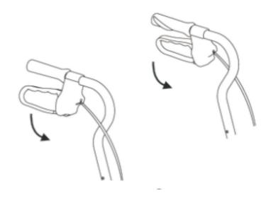
>Upward the hand brake a little bit to remove stop model ;Hang
